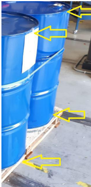
Figure 8. Damage to drums; only face 4.
