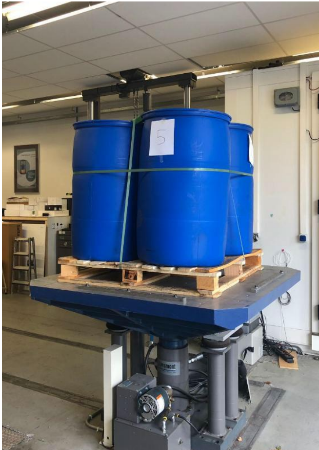
Figure 6. Test setup for vibration test
