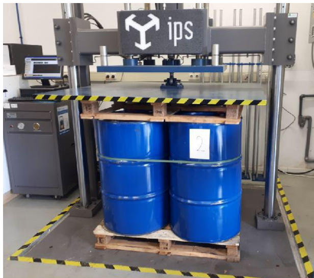
Figure 5. Test set-up Compression Test
