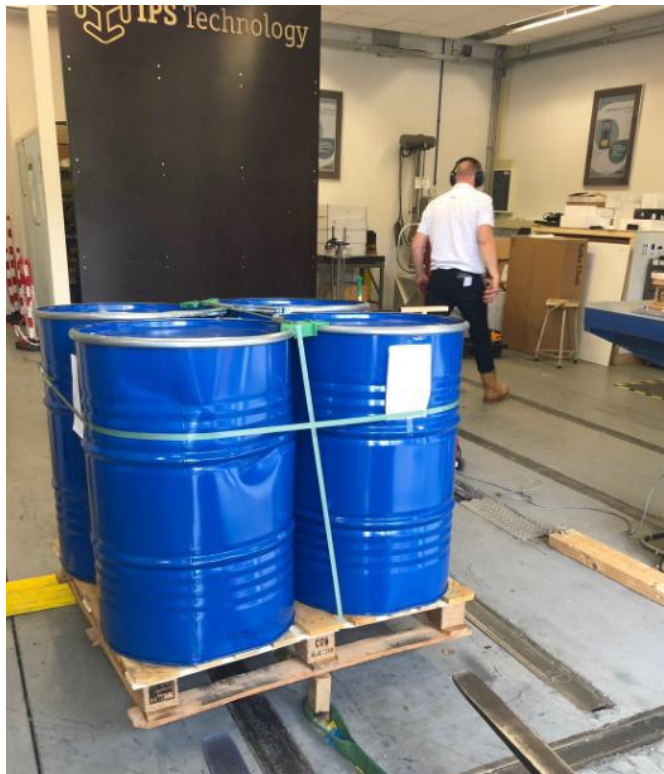
Figure 4. Set-up Rotational Edge Drop Test
