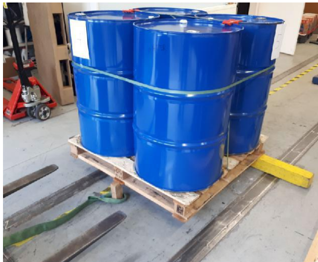
Figure 7. Set-up Rotational Edge Drop Test
