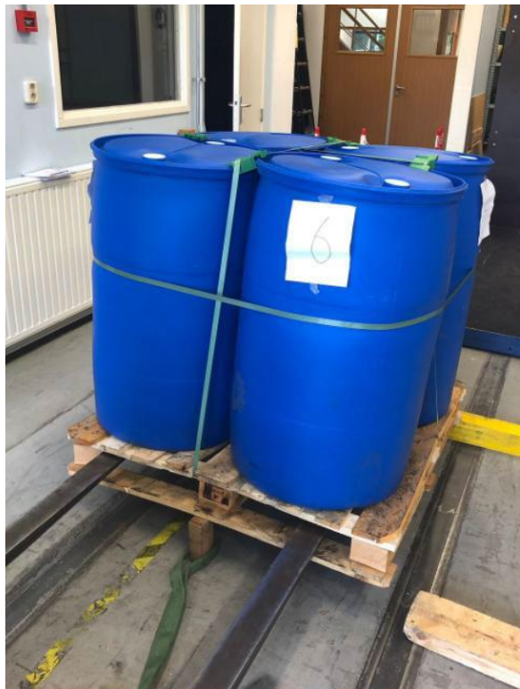
Figure 4. Set-up Rotational Edge Drop Test
