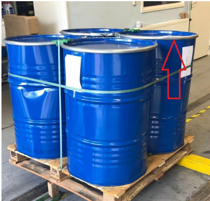
Figure 8. Damage to drum ring; only face 4.
