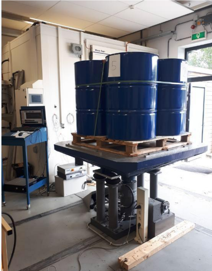
Figure 6. Test setup for vibration test
