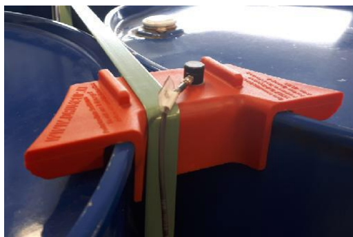
Figure 13. Location accelerometer Ch2. for response monitoring (examination only)
