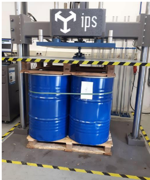
Figure 5. Test set-up Compression Test
