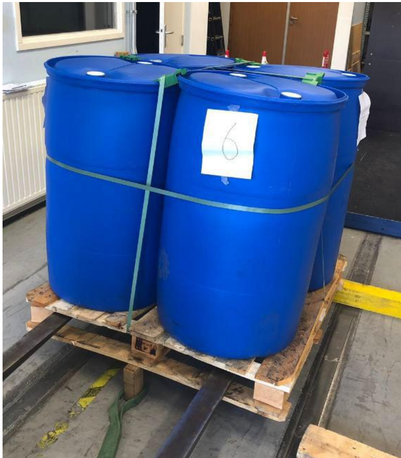
Figure 8. Position of drum clips during drop testing.
