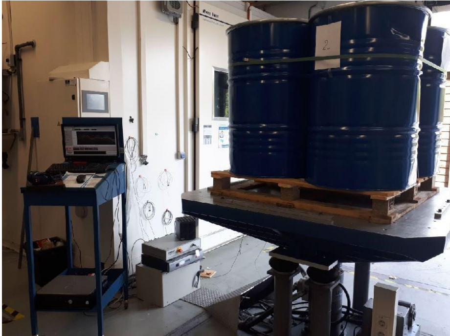
Figure 6. Test setup for vibration test
