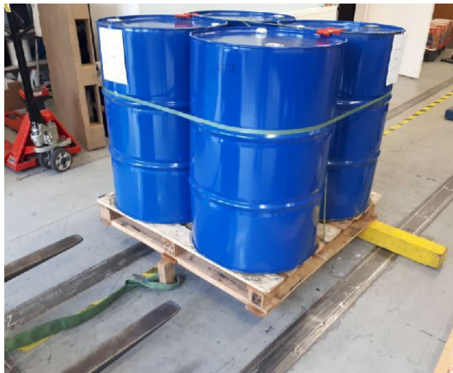
Figure 4. Set-up Rotational Edge Drop Test
