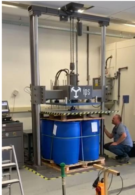
Figure 5. Set-up compression test
