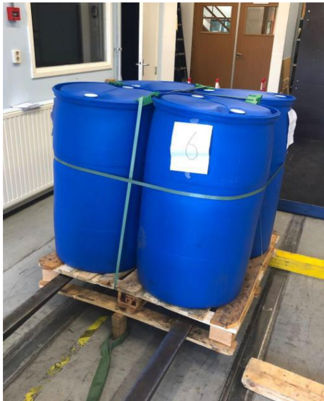
Figure 7. Set-up Rotational Edge Drop Test
