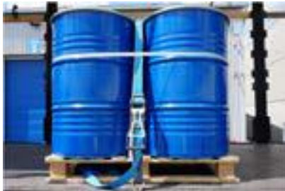
Horizontaler und vertikaler Cordstrap®, Spangurt hinter dem horizontalen Cordstrap® / Horizontal and vertical Cordstrap®, lashing belt behind the horizontal Cordstrap®
