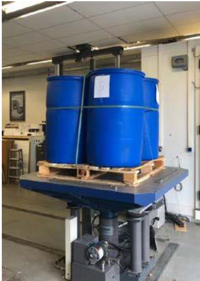
Figure 6. Test setup for vibration test
