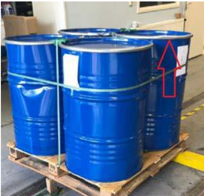
Figure 8. Damage to drum ring; only face 4.
