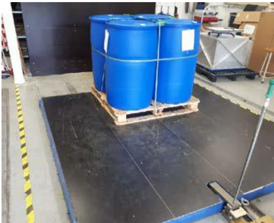
Figure 3.DUT on horizontal impact tester.
