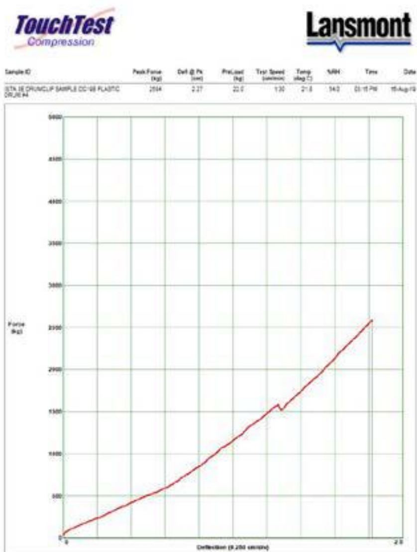
Figure 11. Compression test graph – Apply and release compression test
