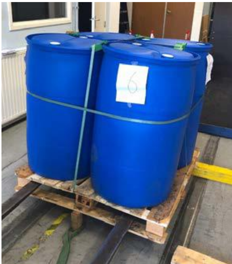
Figure 8. Position of drum clips during drop testing.
