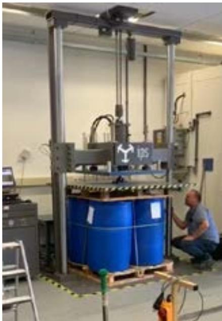
Figure 5. Set-up compression test
