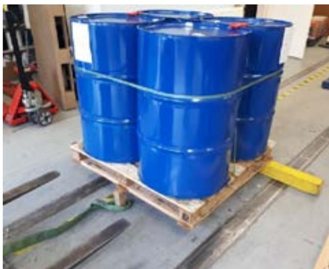
Figure 7. Set-up Rotational Edge Drop Test
