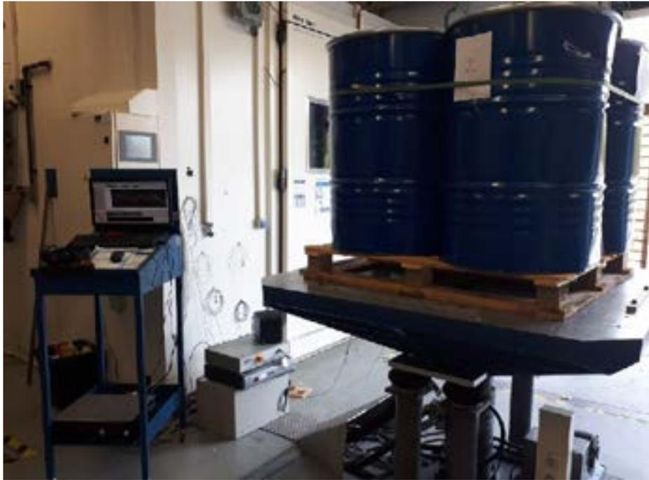
Figure 6. Test setup for vibration test
