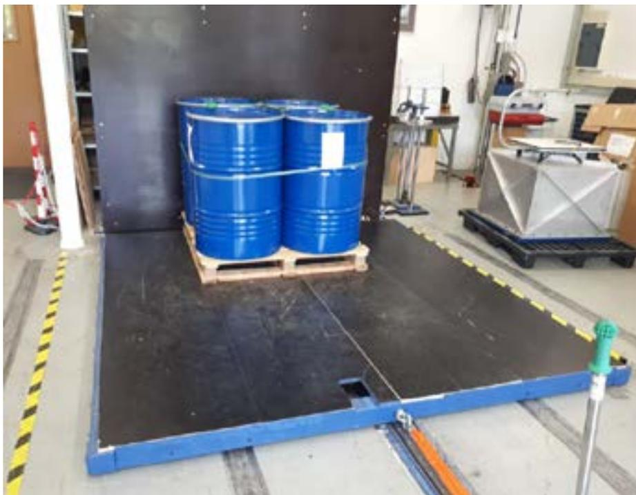
Figure 3.DUT on horizontal impact tester.
