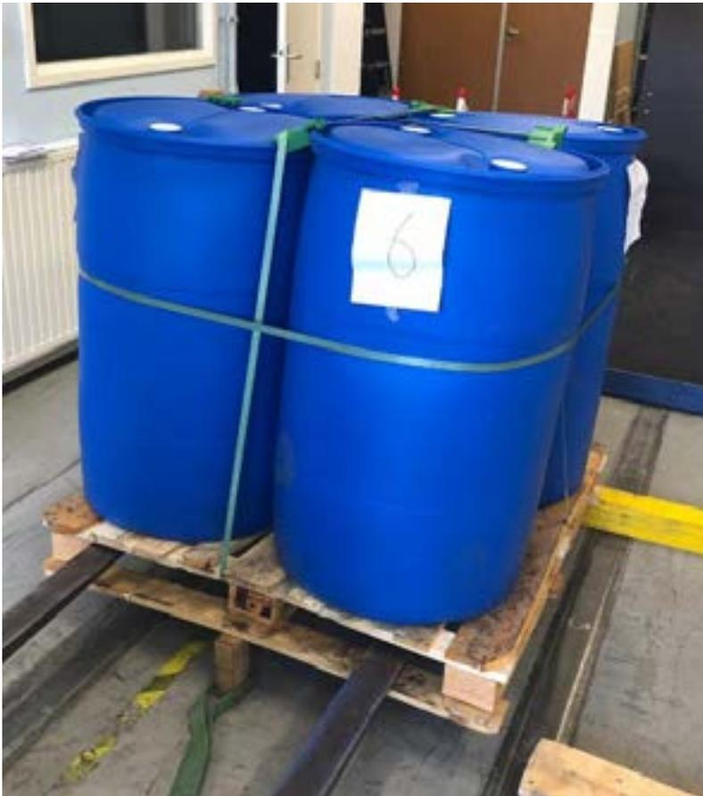
Figure 8. Position of drum clips during drop testing.
