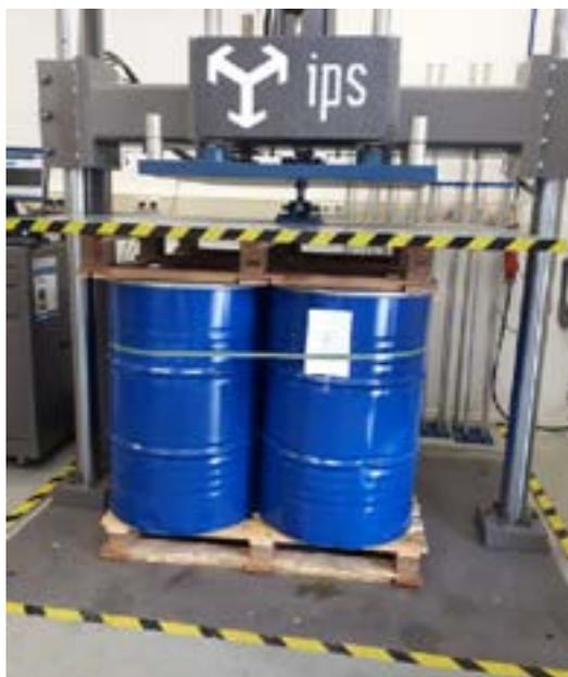
Figure 5. Test set-up Compression Test
