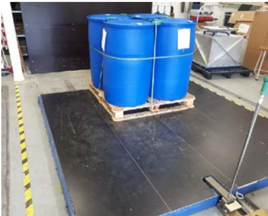
Figure 3.DUT on horizontal impact tester.
