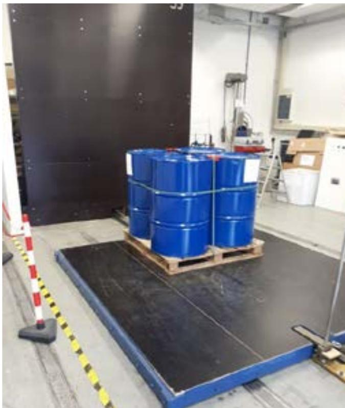
Figure 3.DUT on horizontal impact tester.
