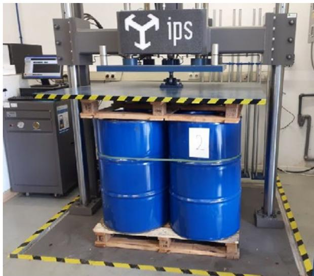
Figure 5. Test set-up Compression Test
