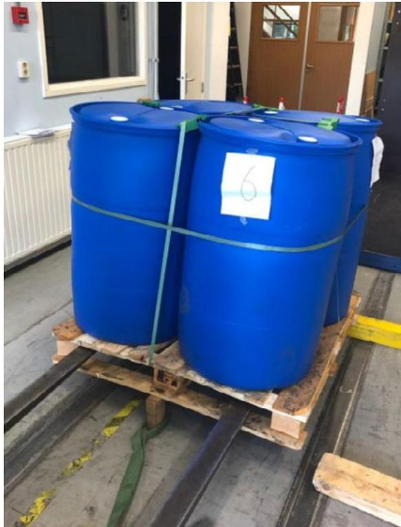
Figure 4. Set-up Rotational Edge Drop Test
