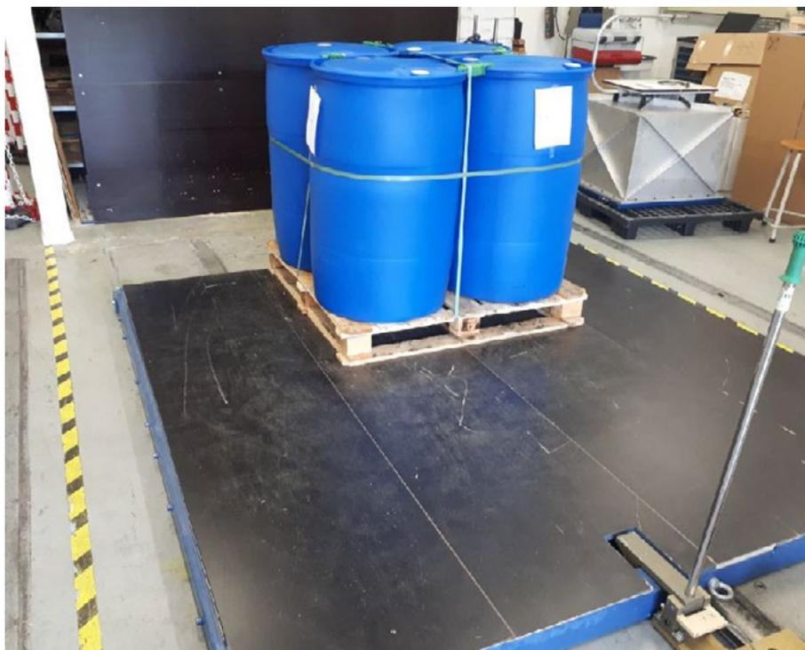
Figure 3.DUT on horizontal impact tester.
