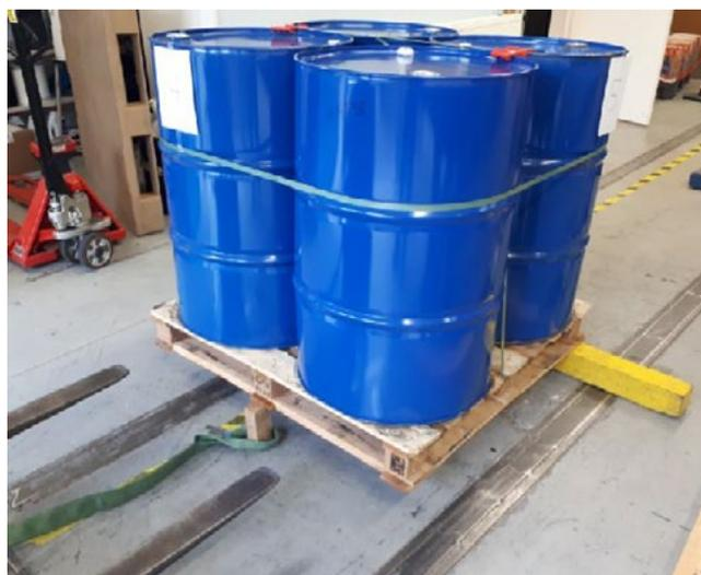
Figure 7. Set-up Rotational Edge Drop Test
