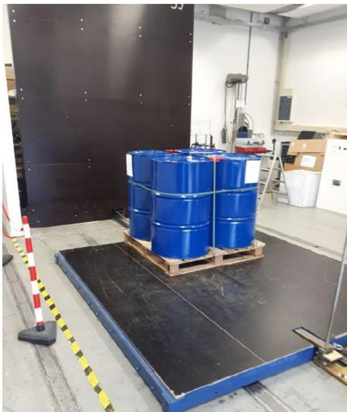
Figure 3.DUT on horizontal impact tester.
