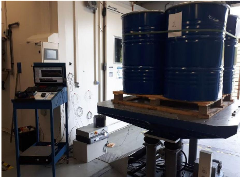
Figure 6. Test setup for vibration test
