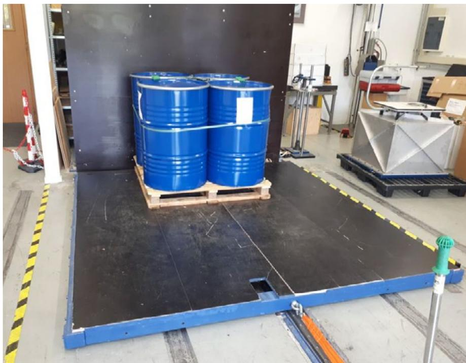
Figure 3. DUT on horizontal impact tester.
