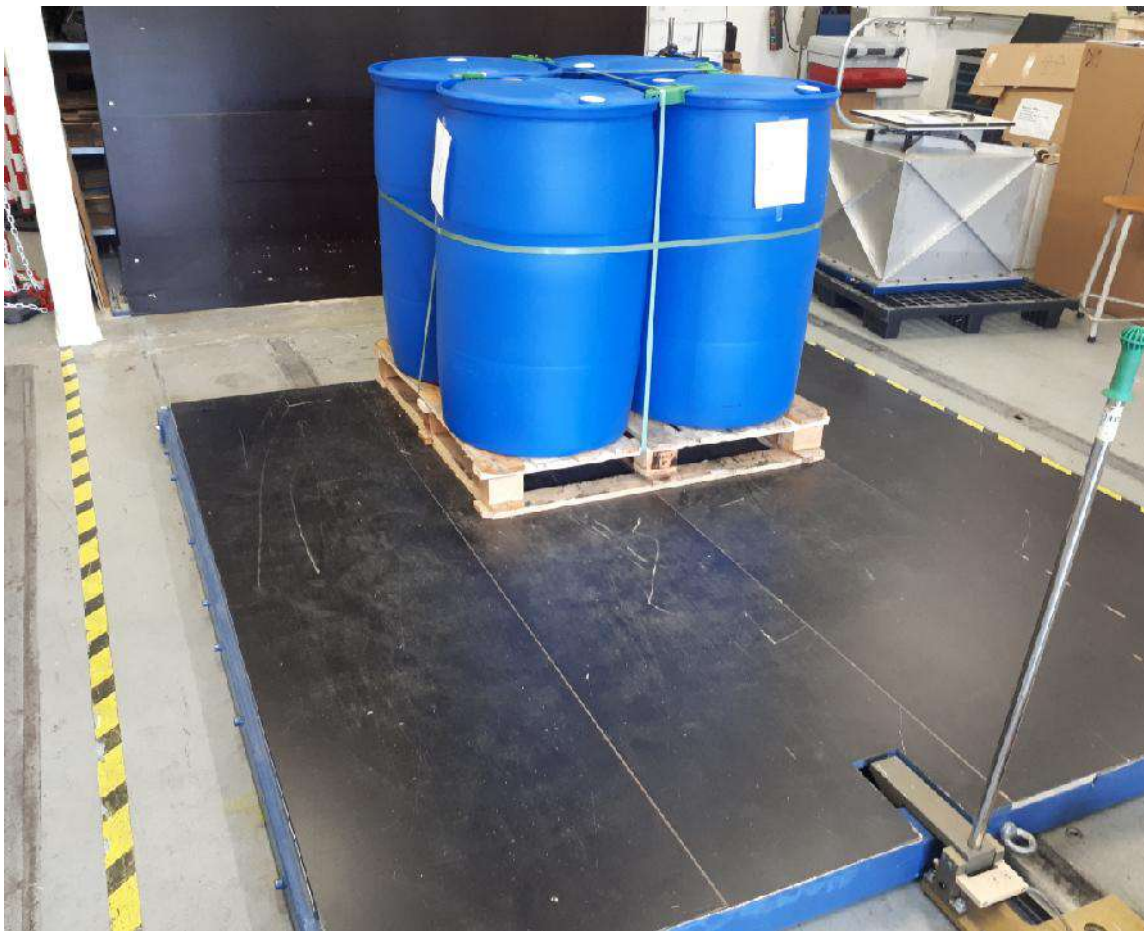
Figure 3.DUT on horizontal impact tester.
