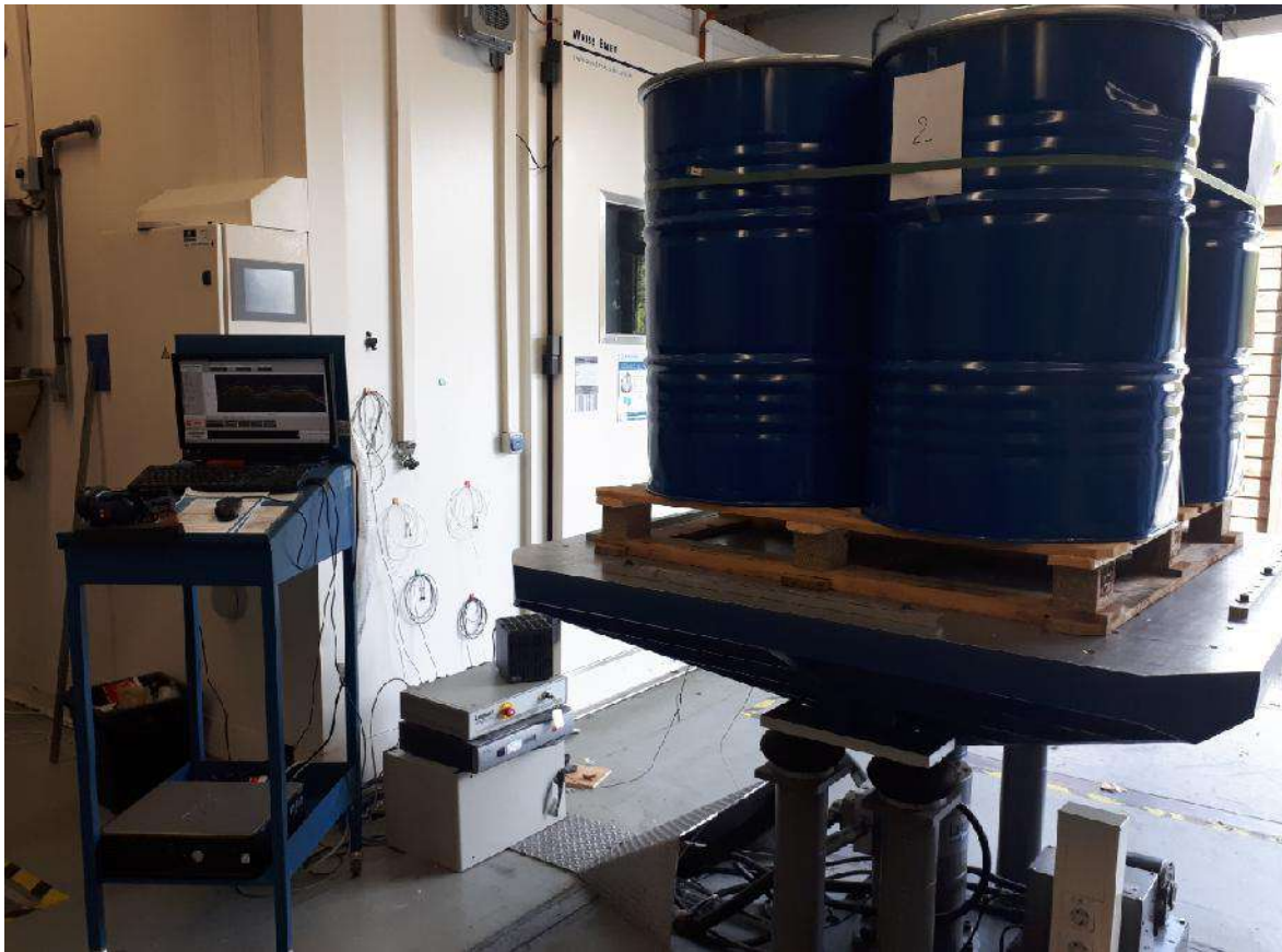
Figure 6. Test setup for vibration test
