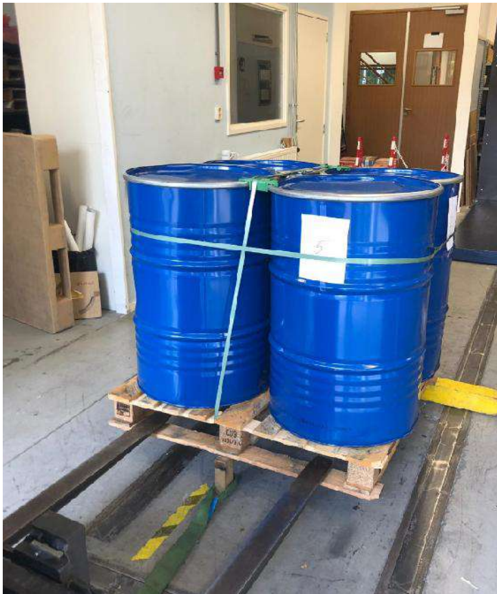
Figure 7. Set-up Rotational Edge Drop Test
