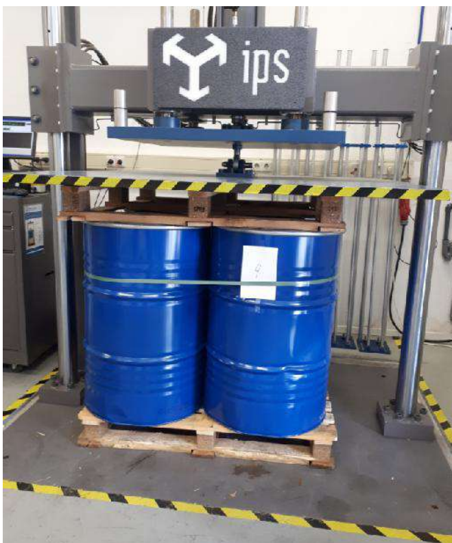
Figure 5. Test set-up Compression Test
