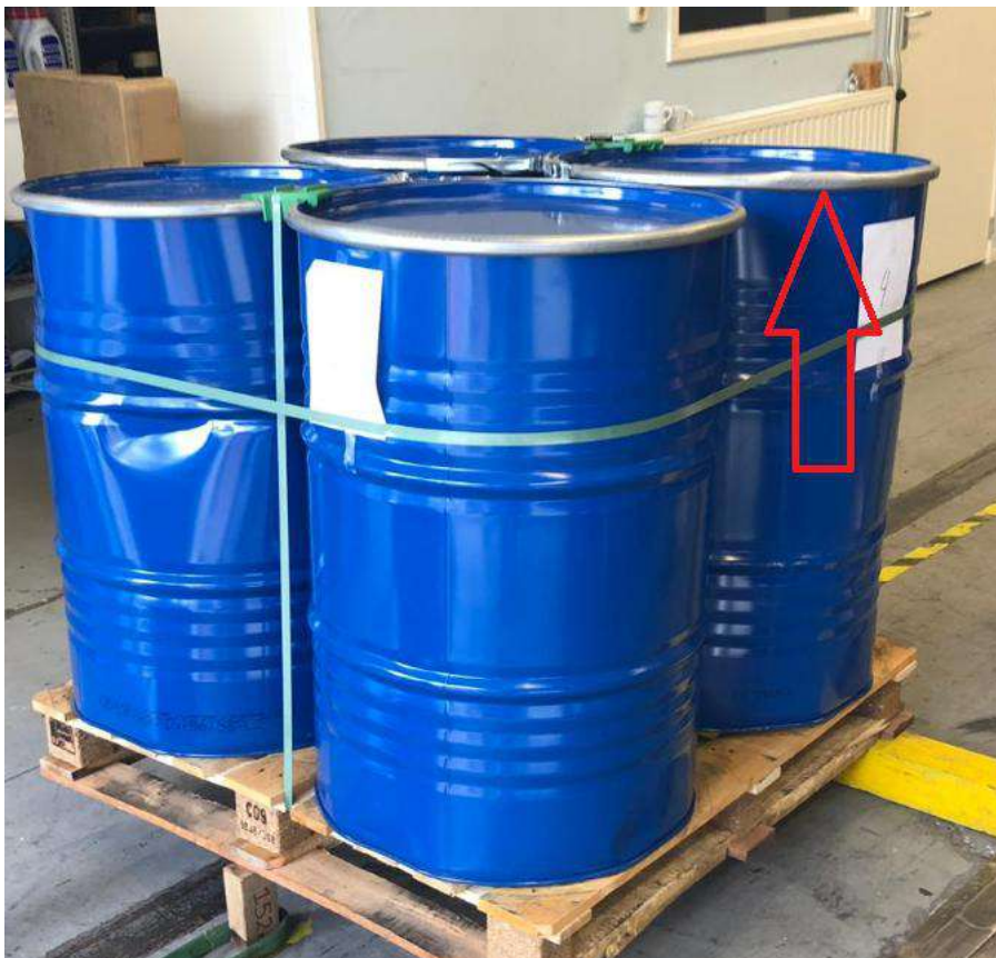
Figure 8. Damage to drum ring; only face 4.
