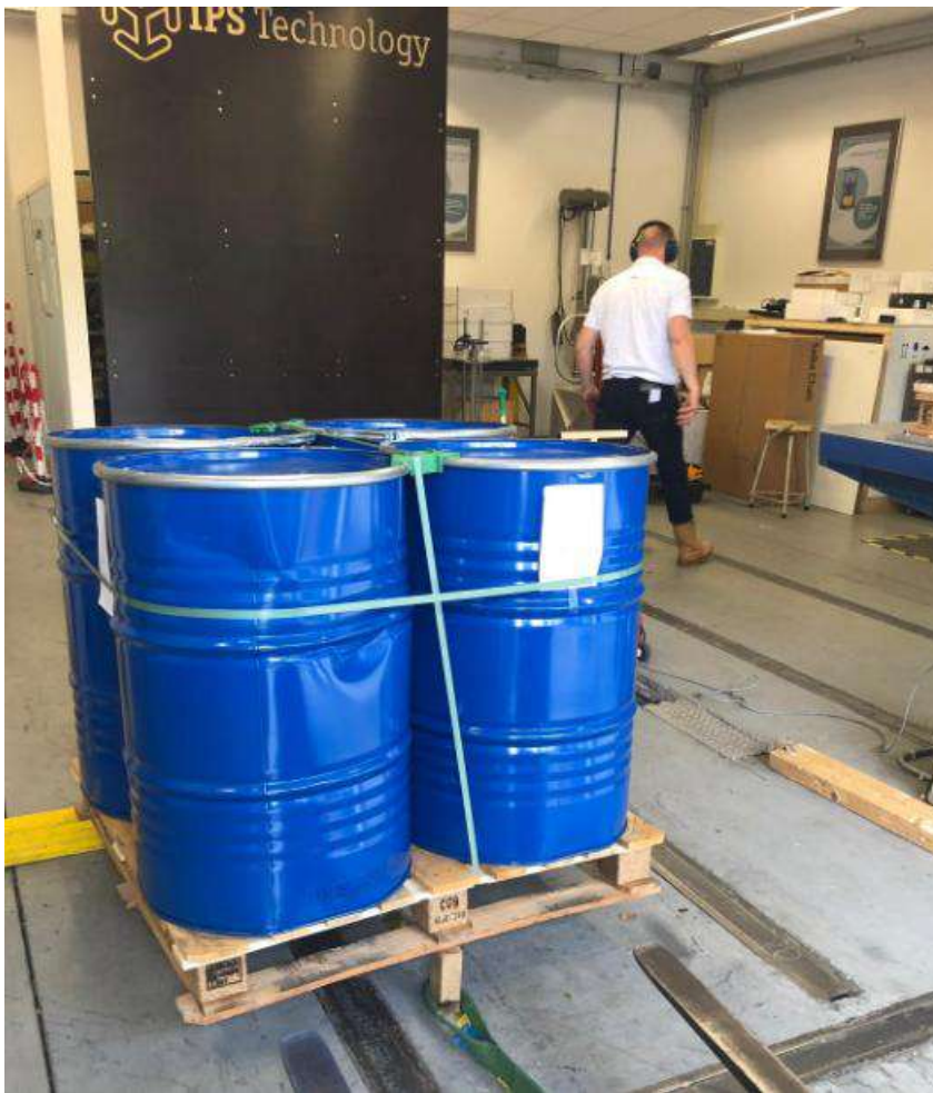
Figure 4. Set-up Rotational Edge Drop Test
