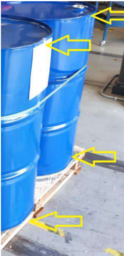
Figure 8. Damage to drums; only face 4.
