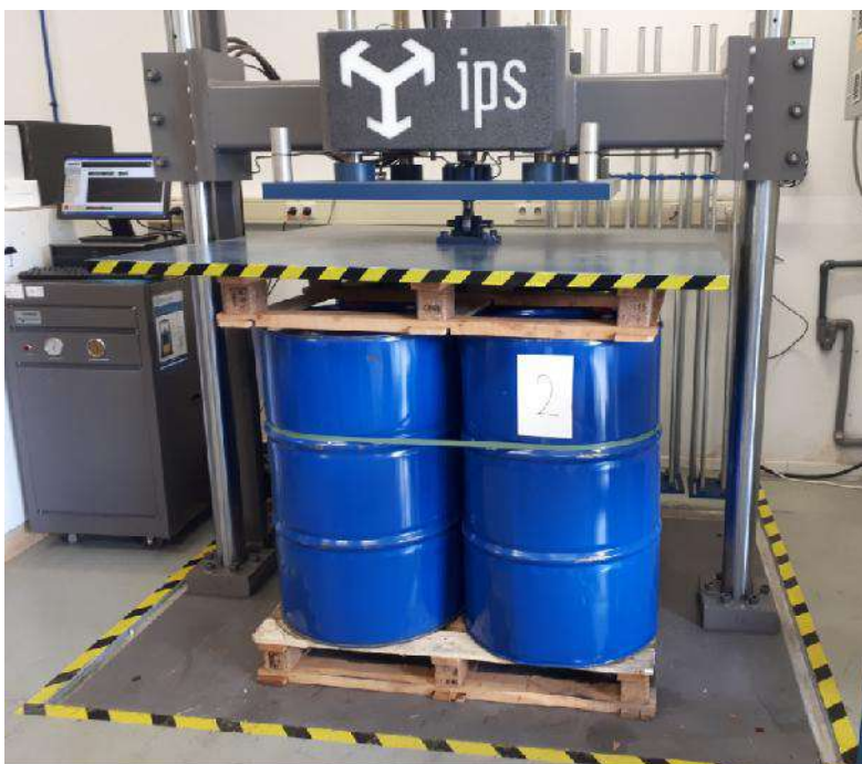
Figure 5. Test set-up Compression Test
