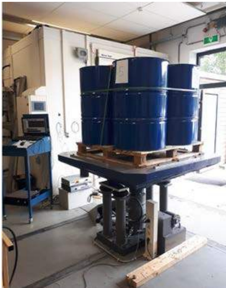
Figure 6. Test setup for vibration test
