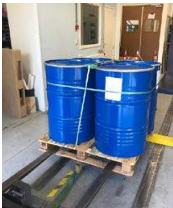
Figure 7. Set-up Rotational Edge Drop Test
