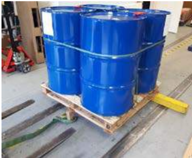
Figure 7. Set-up Rotational Edge Drop Test
