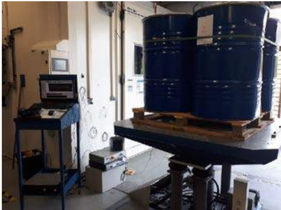
Figure 6. Test setup for vibration test
