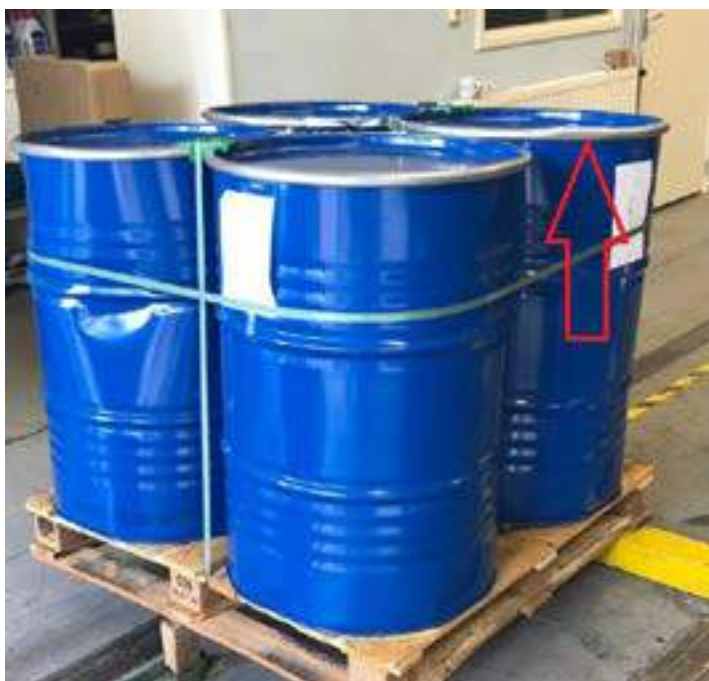
Figure 8. Damage to drum ring; only face 4.
