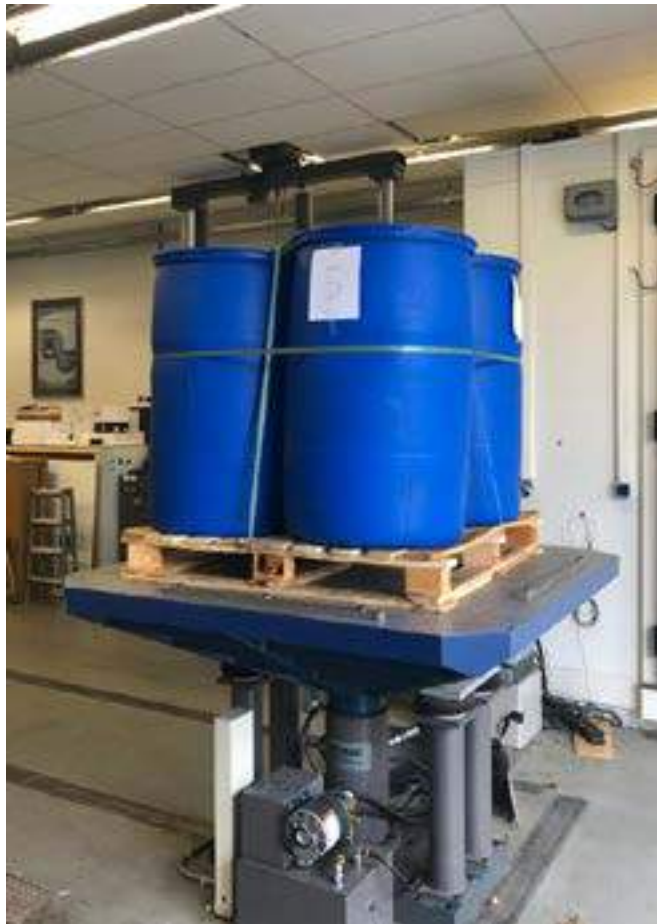
Figure 6. Test setup for vibration test
