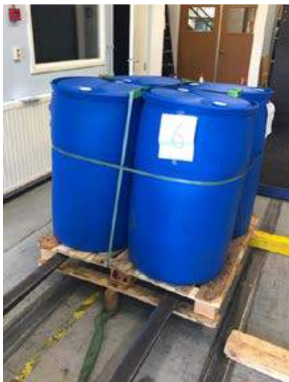
Figure 4. Set-up Rotational Edge Drop Test
