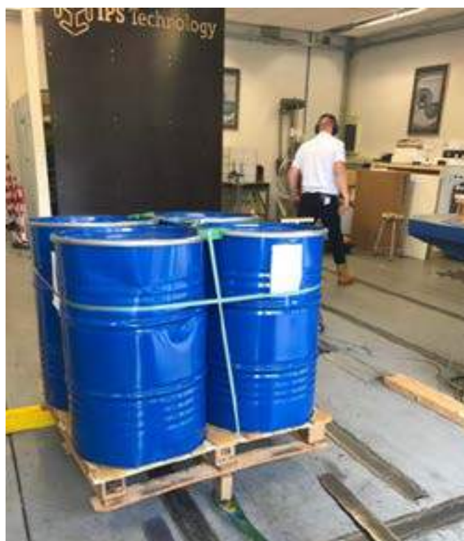
Figure 4. Set-up Rotational Edge Drop Test
