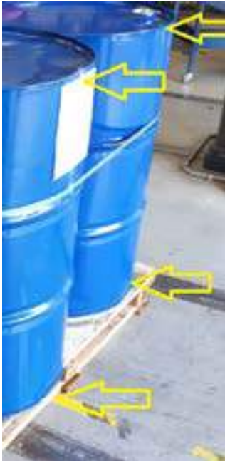
Figure 8. Damage to drums; only face 4.
