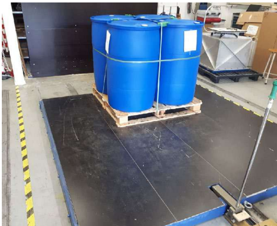
Figure 3.DUT on horizontal impact tester.
