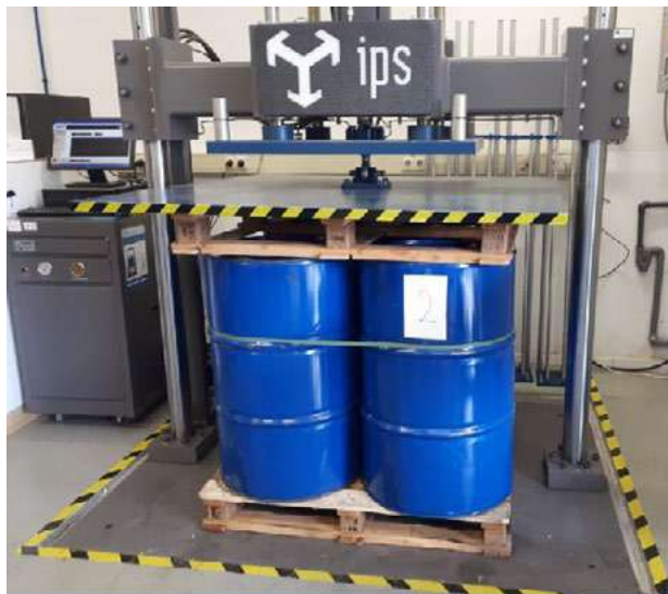
Figure 5. Test set-up Compression Test
