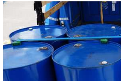
Detailansicht zwei Drumclips pro Ladeinheit / Detailed view of two Drumclips per load unit
