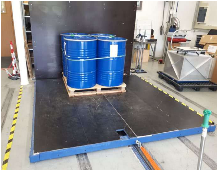
Figure 3. DUT on horizontal impact tester.
