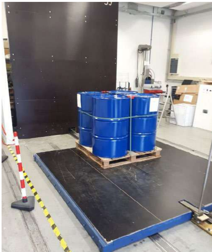
Figure 3.DUT on horizontal impact tester.
