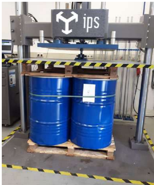
Figure 5. Test set-up Compression Test
