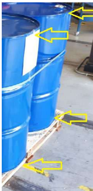
Figure 8. Damage to drums; only face 4.
