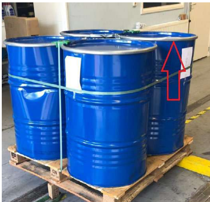
Figure 8. Damage to drum ring; only face 4.
