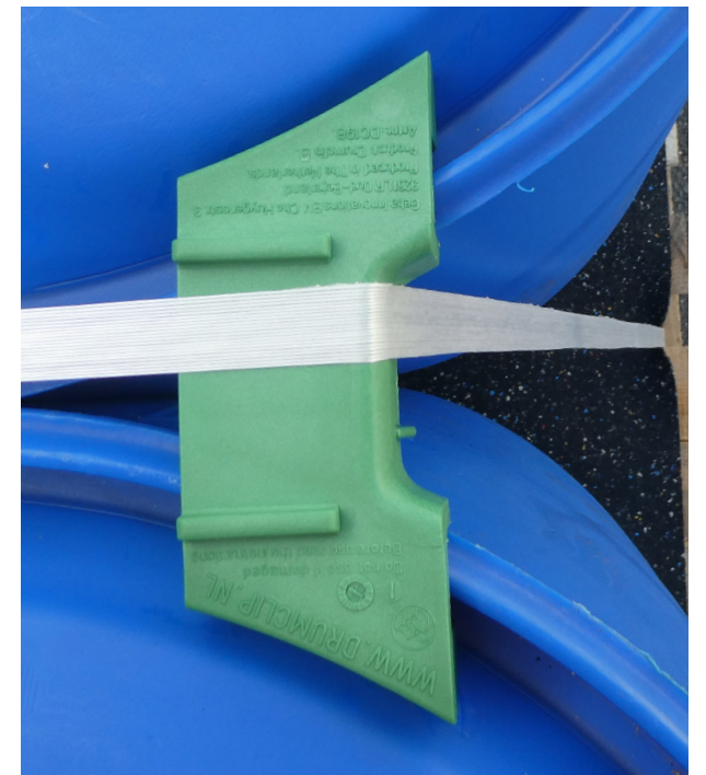
Figure 29: DRUMCLIP DC19B GREEN secured with Cordstrap CC65 & CB6S strap
